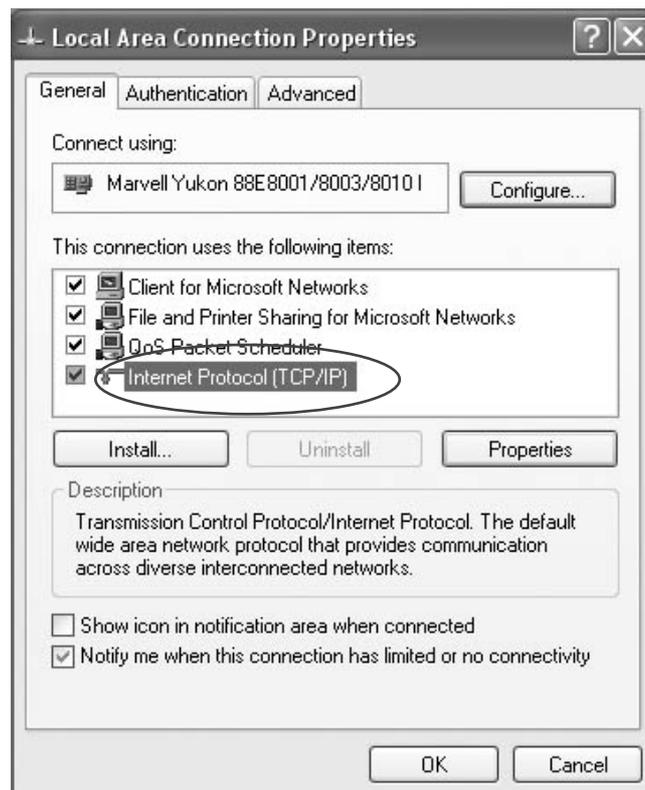
5) As in the Internet Protocol(TCP/IP) Properties dialog box below, choose "Obtain an IP address automatically" and "Obtain DNS Server address automatically" respectively. It completes the PC setup.
