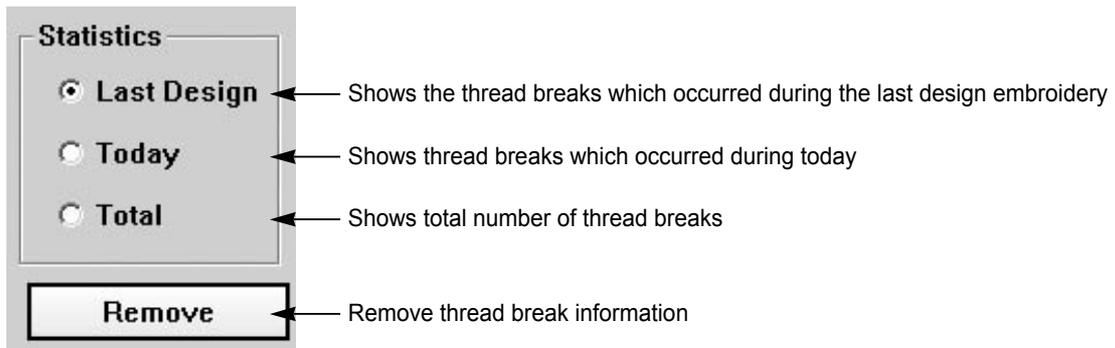
② **Thread Breaks info window** : It shows the thread breaks information by head and needle bar, respectively.
