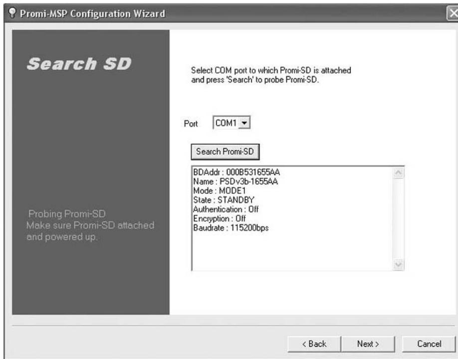
If the search result does not appear, check whether Promi-SD's power is on. Then, press "Reset" button on the side to initialize Promi-SD. Press "Promi-MSP Search" button again for the second trial (check the red LED).
