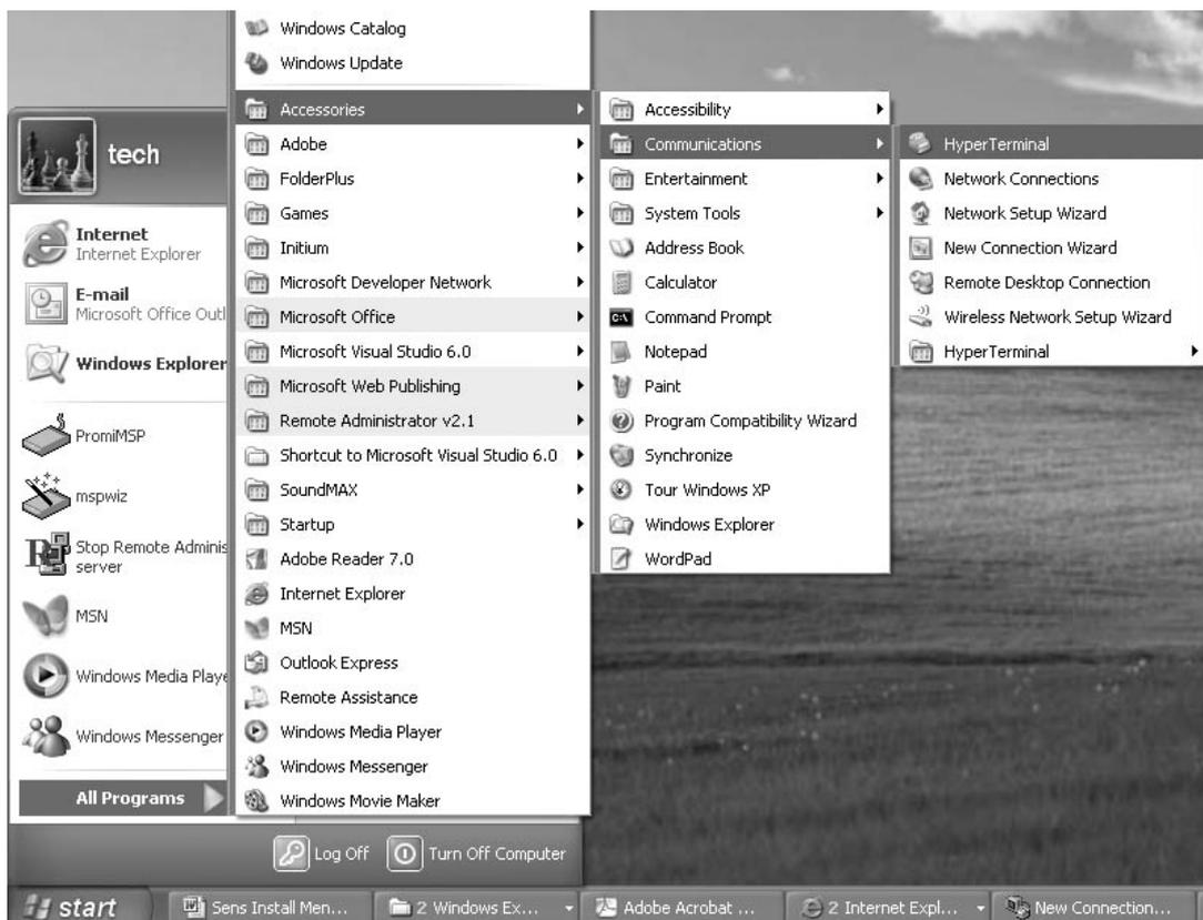
(4) After selecting HyperTerminal, set up COM port as in the below table.
