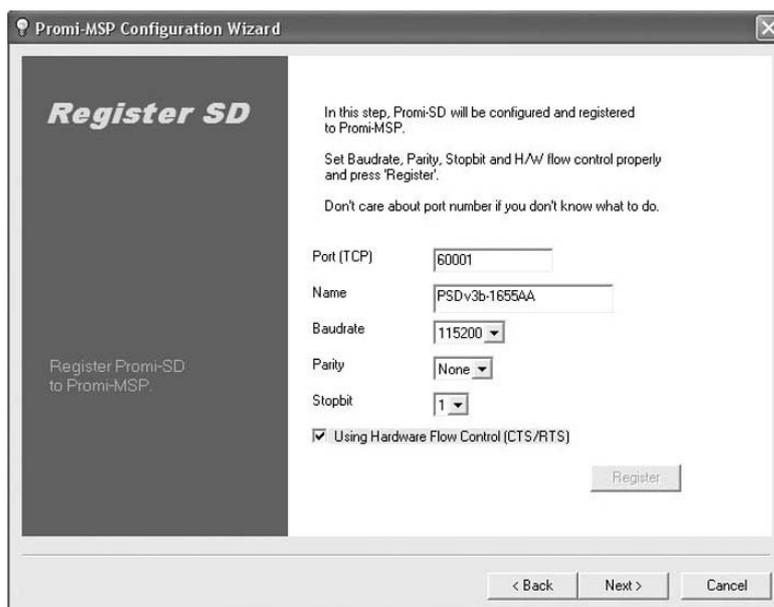
If the setup is made as above, the communication with Promi-SD is conducted through the #60001 TCP port. Promi-SD is set as Mode 1, 115200-8N1-HW. Press "Next" to move to the next step.
