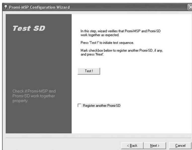
If there are more Promi-SDs to register, check "Register another Promi-SD" at the bottom of the dialog box and then press "Next". It brings the user to the 6th step of Search Promi-SD. Connect the new Promi-SD to the serial port for registration, and repeat the same process again from #6. Press "Next" to complete all settings.
